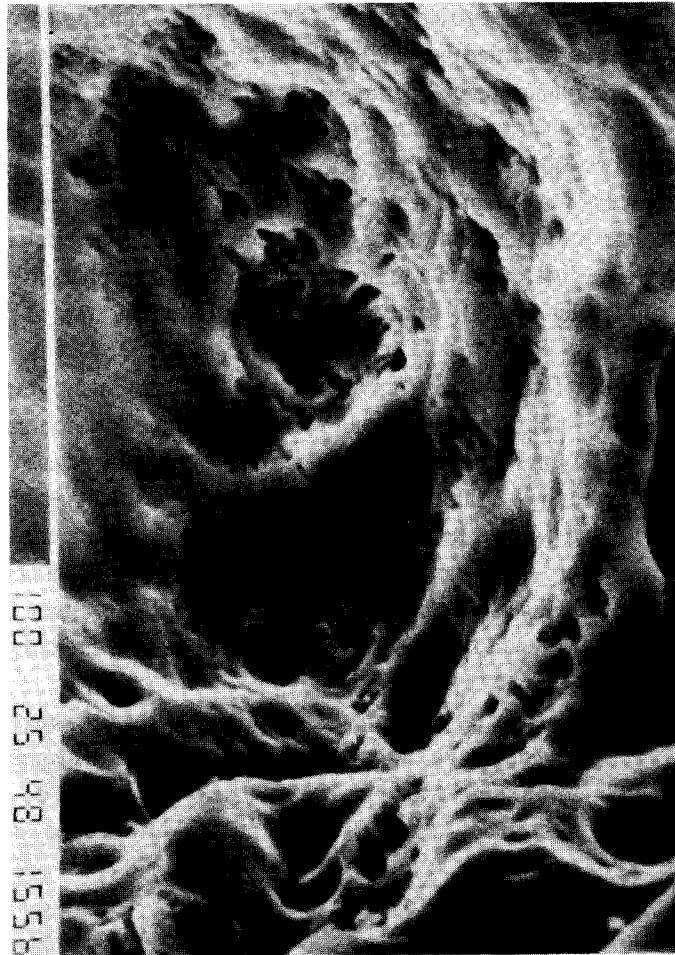
Fig. 3: Microstructure of magnesium in the as-cast condition after the evaluation test, in which it can be observed that the corrosion pattern is by pitting.
