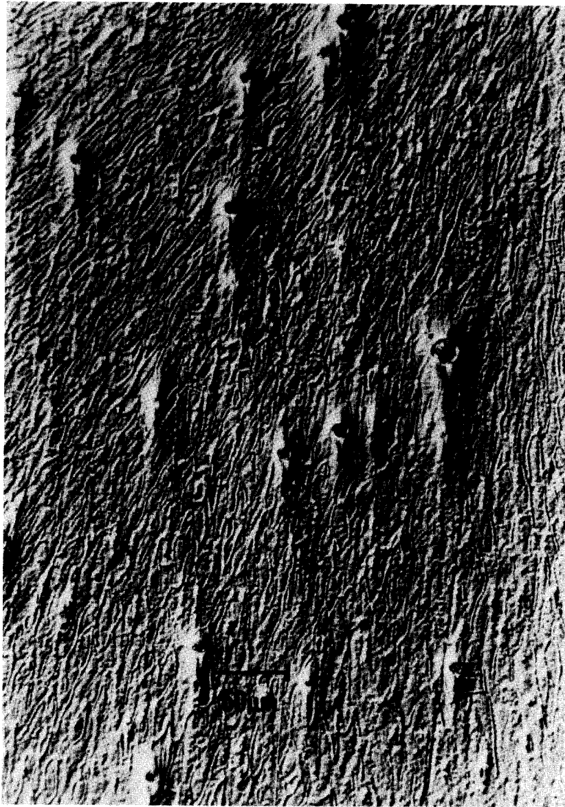
Fig. 1: Cellular microstructure obtained by gravity casting commercial magnesium into a cylindrical copper mould. Second phase particles were detected as Fe-rich particles.
