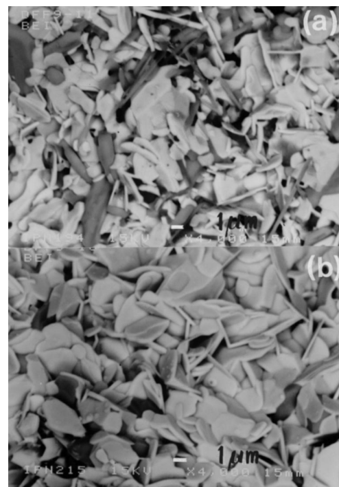
Fig. 5. Surface morphology obtained with backscattered electrons for Bi–Pb–Sr–Ca–Cu–O/MgO films prepared following the experimental conditions of trial nos. 11, (a) and 16, (b) Table 1.
