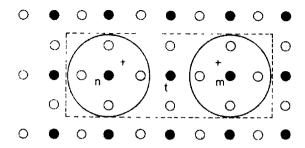
Figure 1. Example of coupled hole pair on the  $CuO_2$  plane in high- $T_c$  superconducting ceramics, black circles are Cu, open circles are O.
