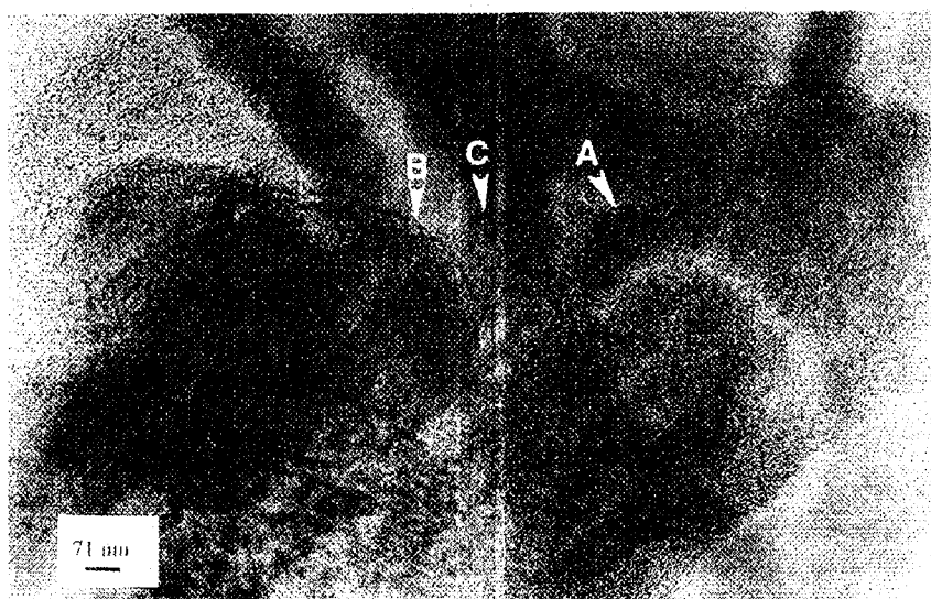
Figure 6. Depicts an electron micrograph of an area where onion-like structures A, and tubular MoSe 2 , B and C are indicated.
