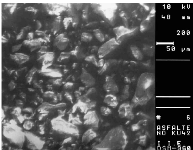
Fig. 1. SEM micrograph of asphaltene particles.
