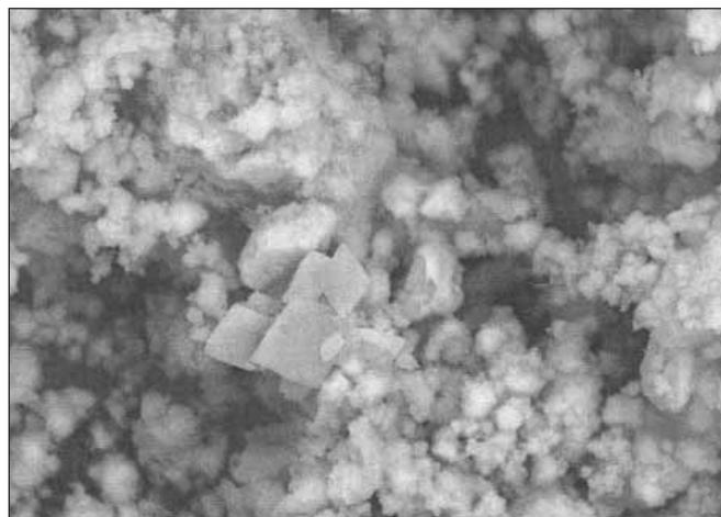
Fig. 1 - Microstructure of the bone cement.
