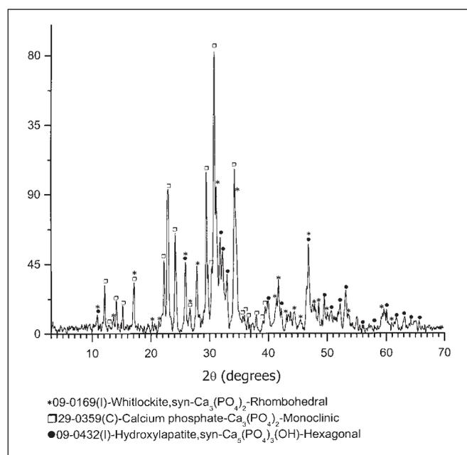
Fig. 2 - Diffraction spectrum of the bone cement.
