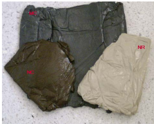
Fig. 1 Photograph showing unvulcanized materials after roll-mill processing. CNR: compounded natural rubber; MC: CNR + FA and NC: CNR + EAFD
