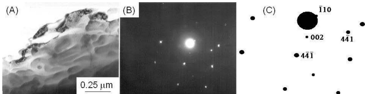
FIGURE 6. (a) TEM micrograph of the \text{Fe}_2\text{Al}_5 intermetallic (b) and (c) diffraction pattern and a key diagram along the [110] axis respectively.
