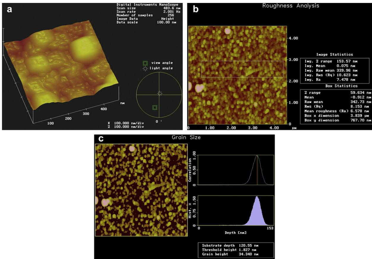
Fig. 6. The AFM images, (a) morphology, (b) roughness and (c) grain size of the film prepared for plasma current,  $I = 0.45$  A,  $\text{Ar}/\text{N}_2 = 60/40$  and  $T = 400$  °C,  $P = 6.0$  mT.
