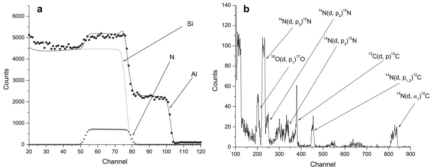
**Fig. 1.** a. The RBS spectrum (low-energy part) arising from elastically scattered beam particles. b. The high energy part containing the peaks from N, O and C nuclear interaction peaks.
