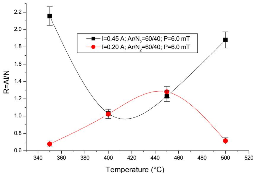
**Fig. 2.** The variation of elemental composition Al/N with substrate temperature for (a)  $I = 0.45$  A and (b)  $I = 0.2$  A,  $T_s = 400^\circ\text{C}$ , Ar/N<sub>2</sub> = 60/40 and  $P = 6.0$  mT.
