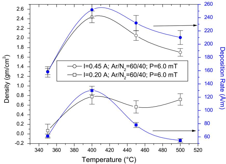
Fig. 3. The variation of (a) deposition rate versus substrate temperature and (b) the density versus temperature for films prepared using  $\text{Ar}/\text{N}_2 = 60/40$ ,  $I = 0.45$  A and  $I = 0.2$  A.
