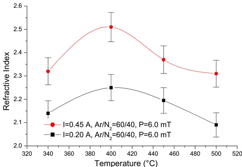
Fig. 5. The variation of refractive index with substrate temperature for the deposition conditions  $\text{Ar}/\text{N}_2 = 60/40$ ,  $I = 0.45$  A and  $I = 0.2$  A.
