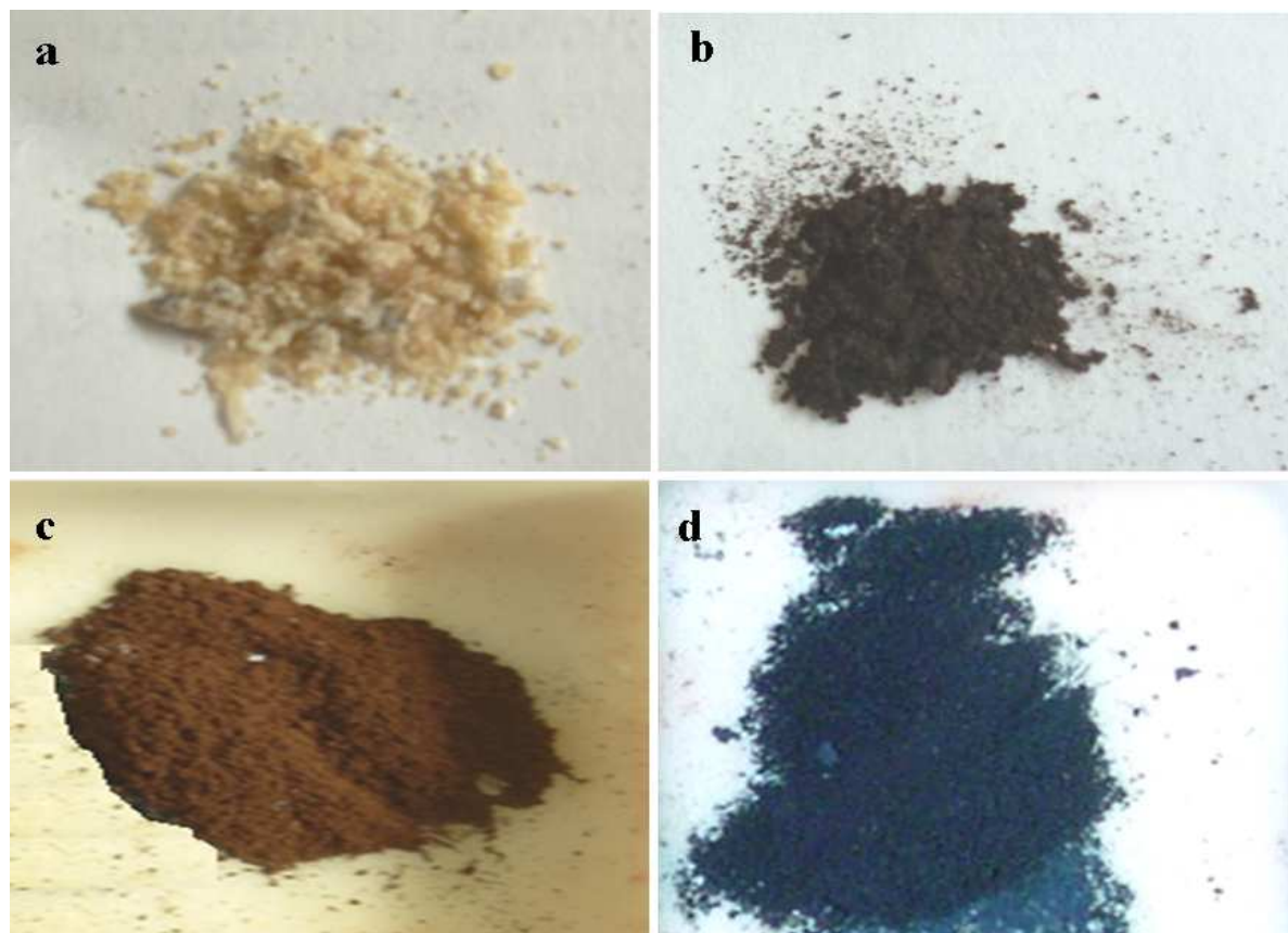
Fig. 1 a ) Dehydrated Pd gel, b ) xerogel, Pd gel after heating up 170 °C c ) Pd sample heated at 600 °C and d ) Pd xerogel powder after a heat treatment at 900 °C.
