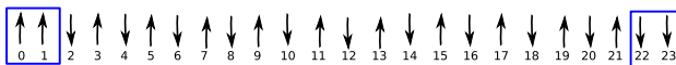
Figure 13. Summary of spin-polarized regions for n = 3/4 as a function of the superexchange coupling J , which causes an alternating polarization to evolve into an antiferromagnetically ordered region.
