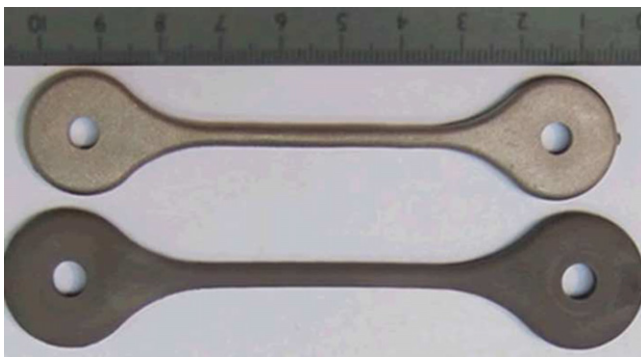
Fig. 11. Photograph illustrating the linear shrinkage undergone by a MIM sintered CP-Ti part.
