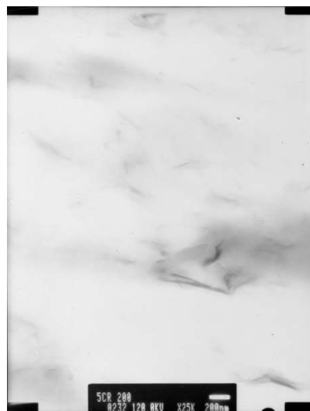
Figure 2 TEM photograph of the 5 phr NC film.
