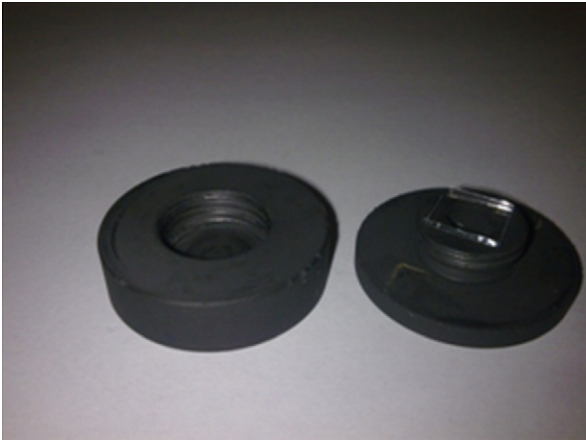
Fig. 1. Semi-closed graphite boat used for the preparation of GaN by close space vapor transport.
