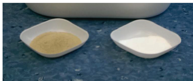
Fig. 7 Photograph of a commercial sample of MIL-53(Al) (left), and our scaled-up material prepared by continuous flow (right).
