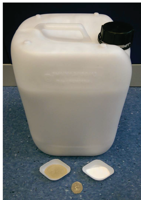
Fig. 6 Photograph of the barrel containing a suspension of MIL-53(Al) formed by continuous flow in our scaled-up reaction (centre), together with a commercial sample (bottom left) and dried MIL-53(Al) from the barrel (bottom right). A fifty pence piece is shown for scale (bottom centre).
