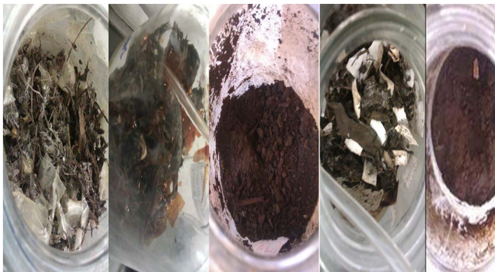
Figure 11. (a) Reactor with MnST-LDPE-Films after 15 days. (b) Reactor with MnST-LDPE-Films after 30 days. (c) Reactor with MnST-LDPE-Films after 45 days. (d) Reactor with cellulose after 7 days. (e) Reactor with cellulose after 45 days. [Color figure can be viewed in the online issue, which is available at wileyonlinelibrary.com .]
