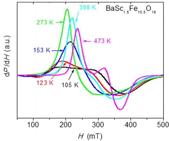
FIG. 4. Electron spin resonance of  $x = 1.5$  sample as a function of temperature. The microwave frequency is 9.43 GHz.
