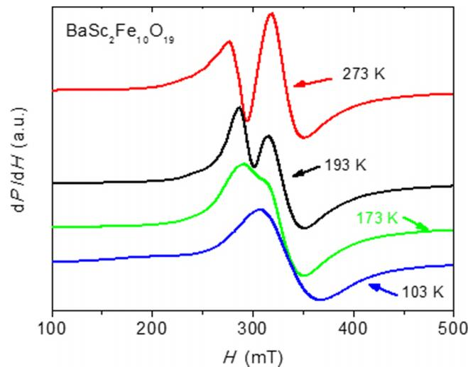
FIG. 5. ESR signals for  $x = 2$  sample, in the low temperature range.
