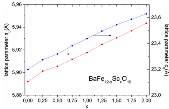
FIG. 2. Lattice parameters vs. Sc concentration for  $\text{BaSc}_x\text{Fe}_{12-x}\text{O}_{19}$ .
