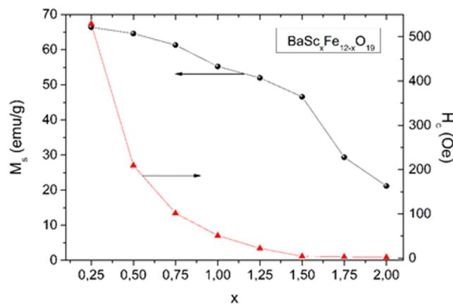
FIG. 3. Saturation magnetization and coercive field at room temperature as a function of the Sc substitution.
