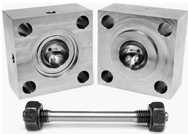
Fig. 2. Connection blocks with large inner volume to reduce dynamic pressure effects.
