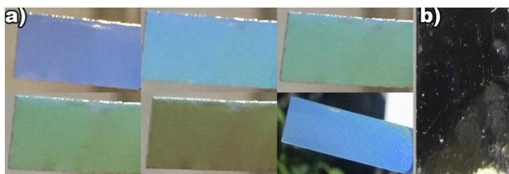
Fig.4. Colored appearance of samples anodized with a) phosphoric acid for different angles and b) oxalic acid.
