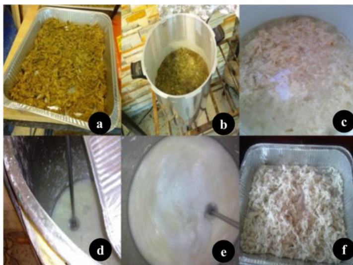
Fig. 1. Cazaurang method: a) Pretreatment, b) Hydrolysis, c) Chlorination, d) Alkaline extraction, e) Whitening, f) Cellulose obtained.
