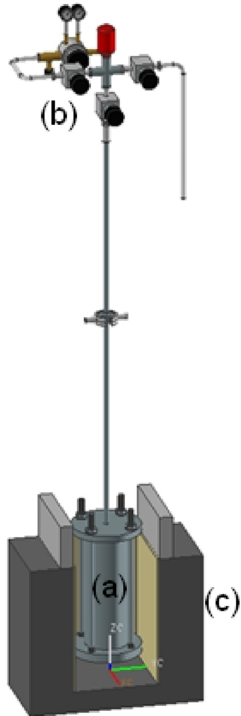
Fig. 1. Replication casting device: (a) steel reaction chamber sealed with two covers, (b) valve system and (c) heating system (furnace).
