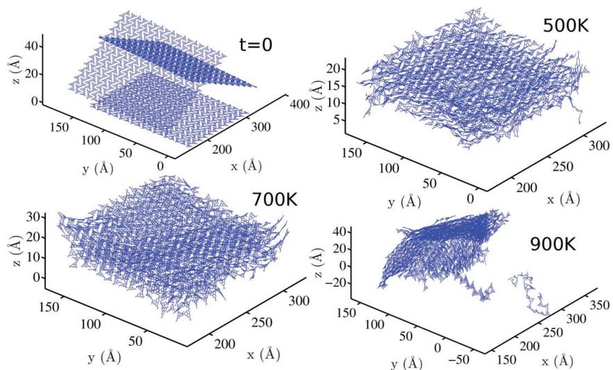
**Figure 4.** Initial ( $t = 0$ ) and equilibrium final trajectory states at different temperatures after the evolution of three sheets in the canonical ensemble.
