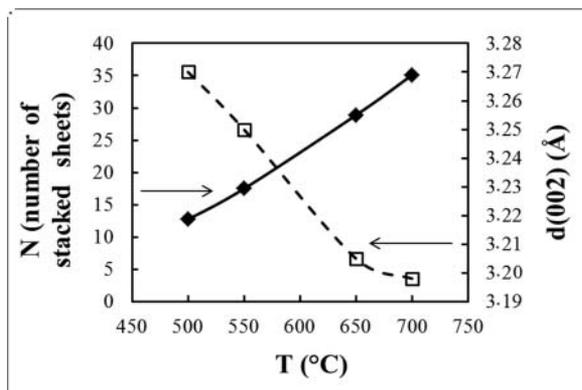
Figure 8. Variation of the interlayer distance and stacked sheets as a function of the synthesis temperature.<sup>[19]</sup>
