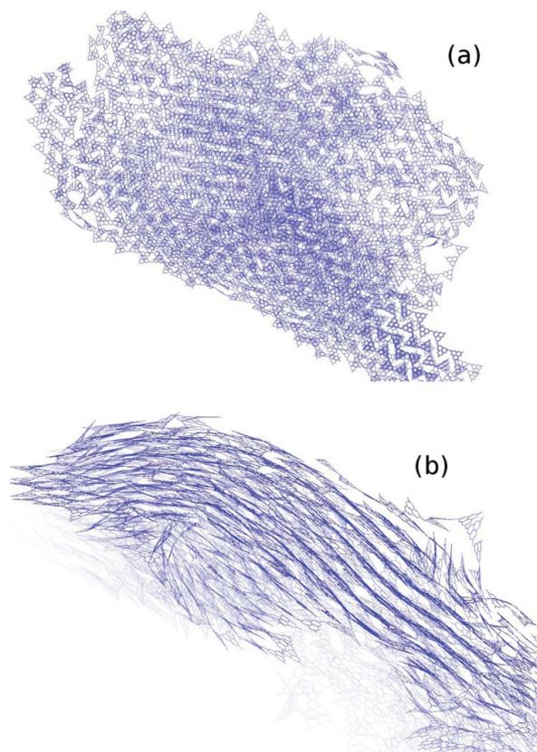
**Figure 5.** A flake obtained by annealing the final equilibrium geometry after evolution in the canonical ensemble at 900 K starting from six sheets of polymeric carbon nitride. (a) top view, (b) side view of the flake edge.
