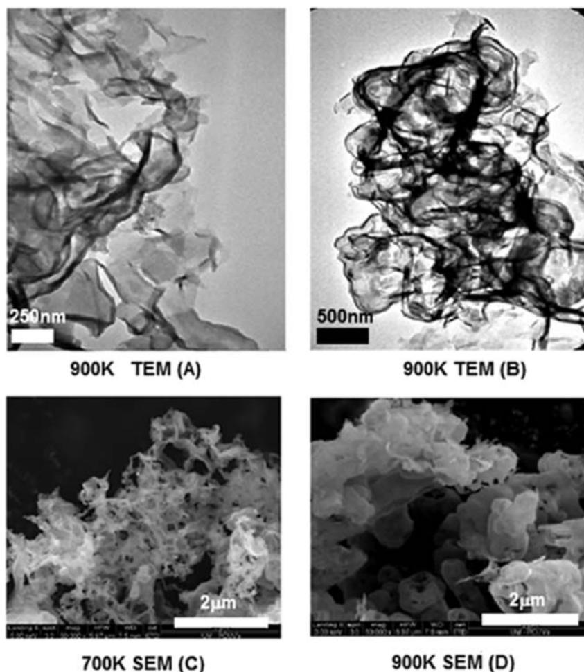
Figure 7. TEM and SEM images of polymeric carbon nitride obtained at 700 and 900 K from melamine cyanurate pyrolysis.
