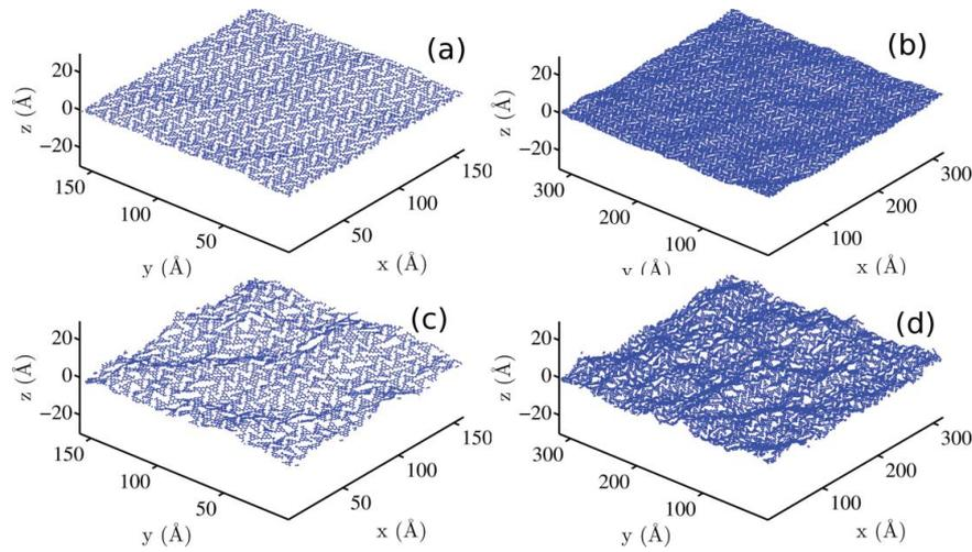
**Figure 1.** Equilibrium polymer sheets at zero pressure obtained using periodic boundary conditions. Left column results ((a) and (c)) correspond to a period of  $13 \times 9$  unit cells; right column ones ((b) and (d)) correspond to a period of  $26 \times 18$  unit cells. Top row results ((a) and (b)) are for a temperature of  $T = 100\text{K}$  and lower row ones ((c) and (d)) for  $T = 700\text{K}$ .
