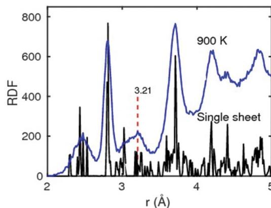
**Figure 6.** Radial distribution function computed for flake depicted in Figure 5 and for a single sheet of material at low temperature.
