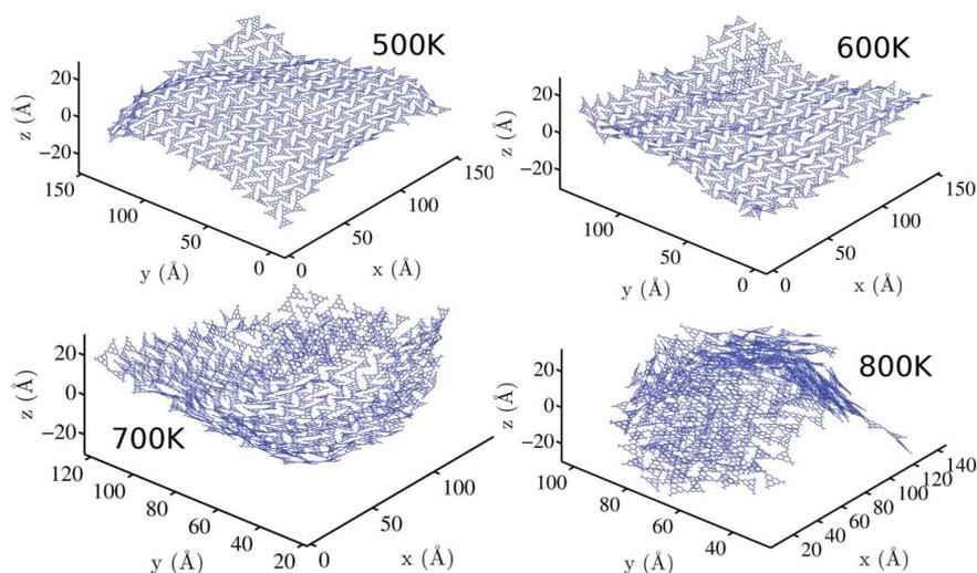
**Figure 3.** Final trajectory states after 500 psec evolution in the NVT ensemble at different temperatures. The initial condition in all cases is a ground state, approximately square, sheet spanning over  $13 \times 9$  unit cells of the 2D polymer.
