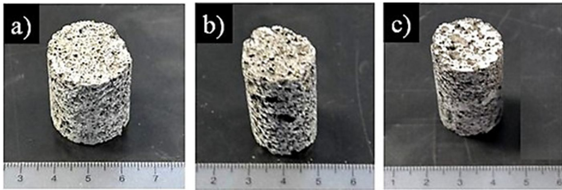
Fig. 2. A356 aluminum alloy foams manufactured to the foaming additions of (a) 1 wt % CaCO 3 , (b) 2 wt % CaCO 3 and (c) 3 wt % CaCO 3 .
